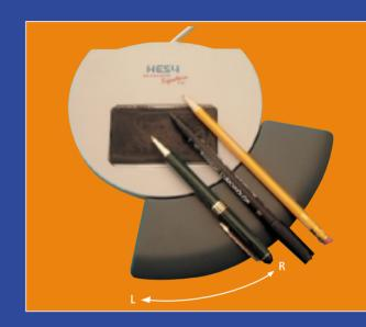
The HESY writing area is a tablet that has four pressure sensors underneath it. It is a form of "writing scales" that records and evaluates all the dynamics of the handwriting. The movable hand rest makes it suitable for both left-handed and right-handed persons.
